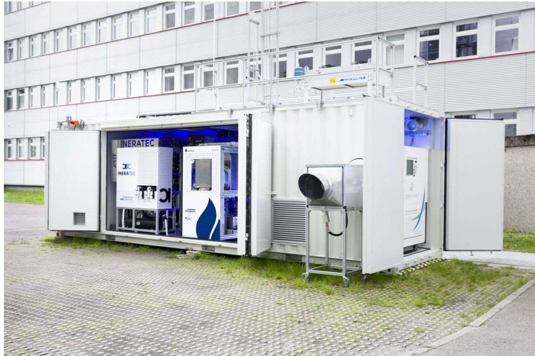
Pilot plant, 10 L/day: https://www.kit.edu/kit/english/pi_2019_107_carbon-neutral-fuels-from-air-and-green-power.php
