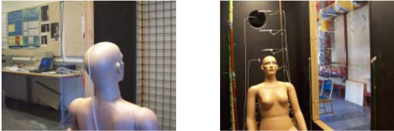
Figure 2. The manikin was positioned centred inside the tunnel with the arms hanging down and no clothing or hair. To the left a view thru the window and towards the front inlet and to the right the manikin and one of the two exhausts for recirculation of the air.
