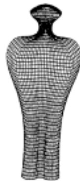
Computational Thermal Manikin Murakami et. al. (1997)
