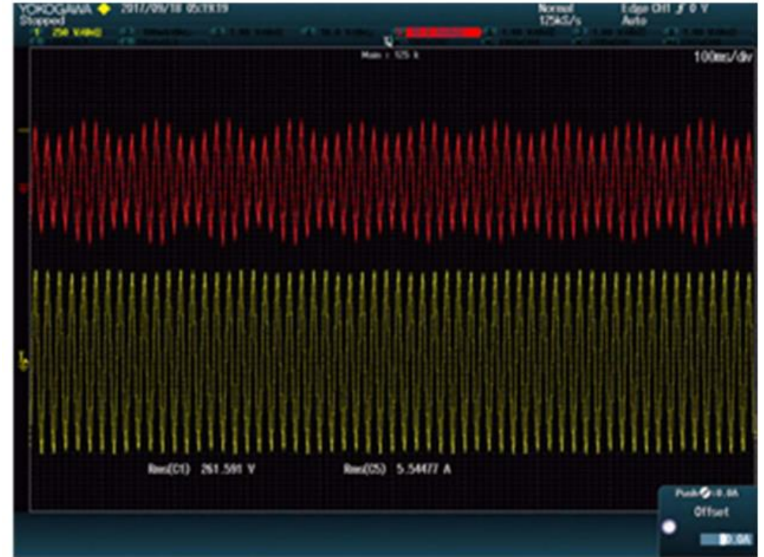
Fig. 1. Measured one PFC converter input current (upper) and voltage (lower) during a data center power system resonance.
