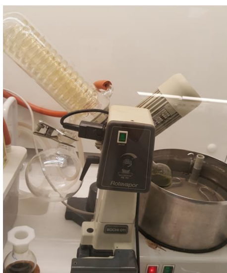
Figure 30 - Evaporation of hexane using a rotary evaporator.
