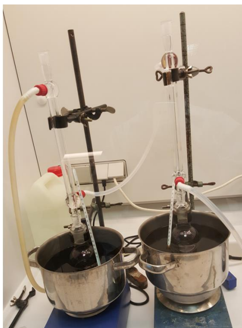
Figure 28 - Lipid extraction with hexane using reflux.
